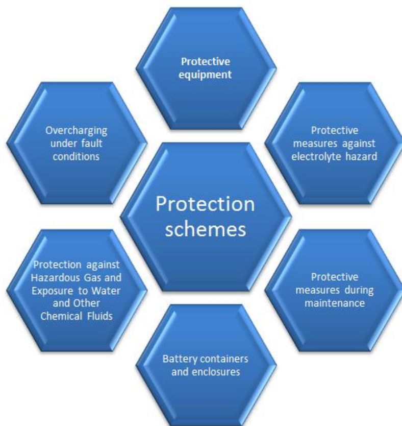
Fig. 3 Required protection schemes inside a battery pack.
